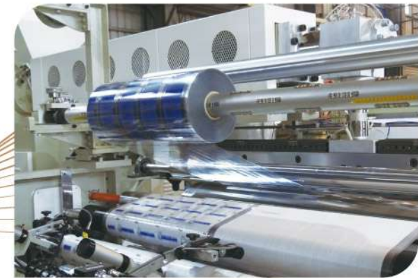
Applicable for Lamination of BOPP Film with PP Woven Bag.
