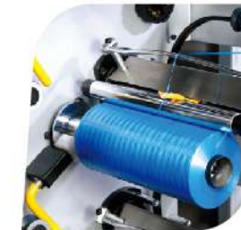
Electronically controlled yarn tension
